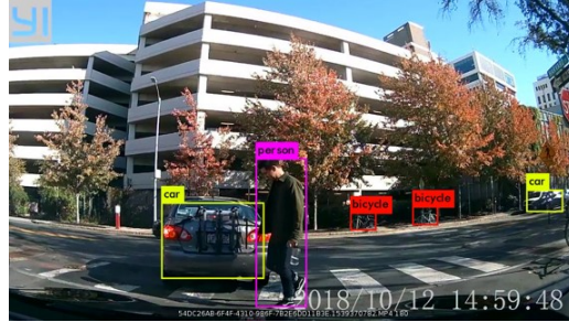
Fig. 5. Result of applying the pre-trained neural network to the Cambridge dataset.
