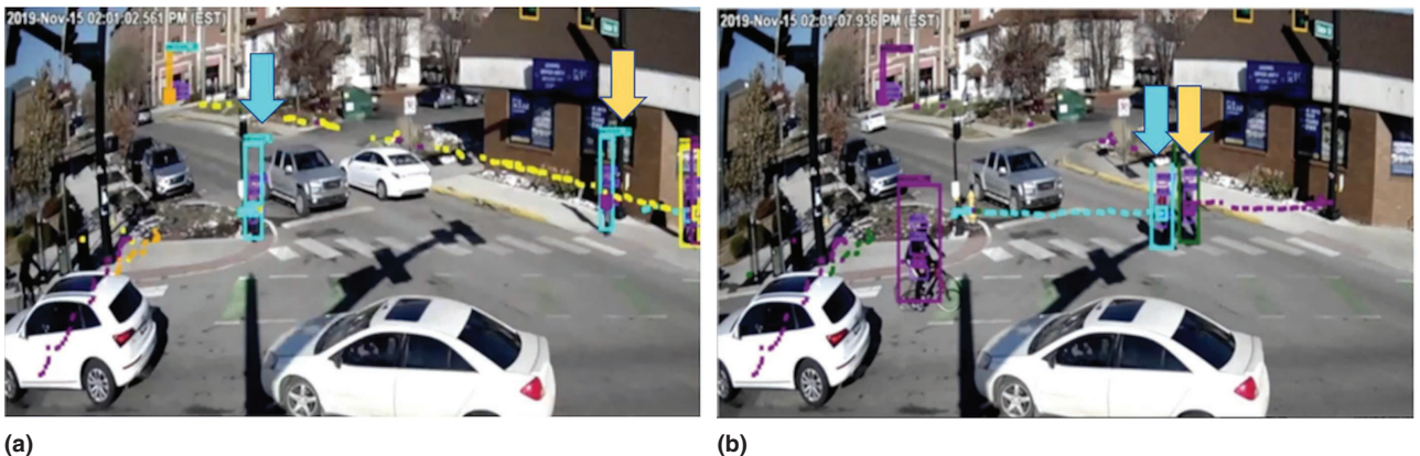
FIGURE 7. The tracking from a single camera of a pedestrian crossing the street at (a) 2:01:02 p.m. and (b) 2:01:07 p.m.
