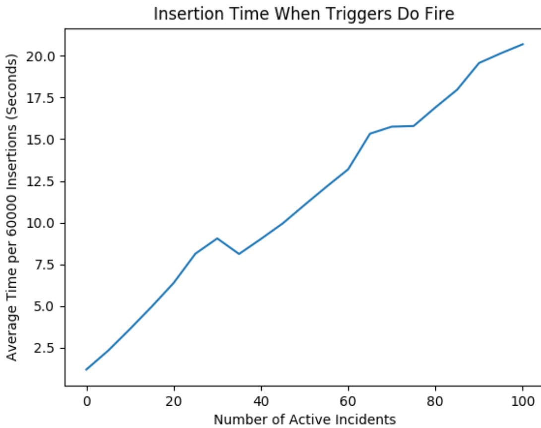
Figure 2.14. Insertion Time vs Number of Trigger Functions. Insertion times are calculated on an average of 5 trials.
